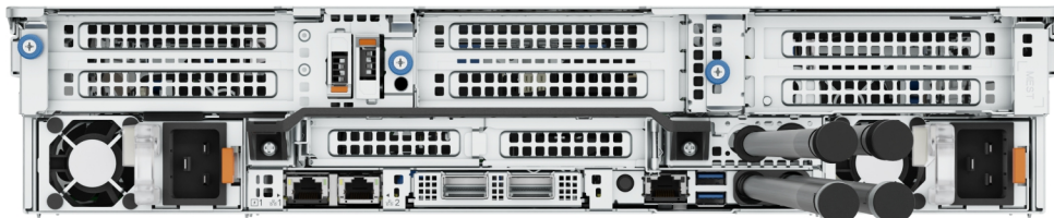
Figure 8. Rear view of the system with Direct Liquid Cooling
