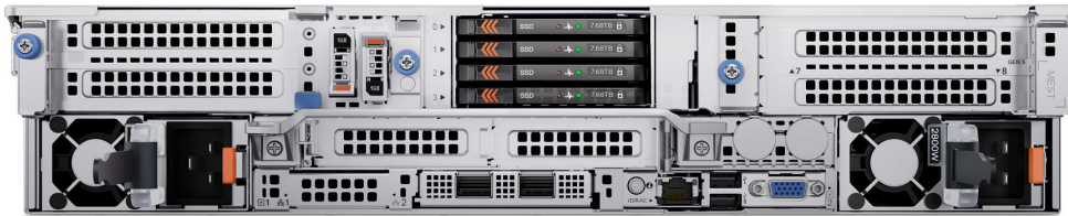
Figure 7. Rear view of the system with 4 x EDSFF E3.S drive system
